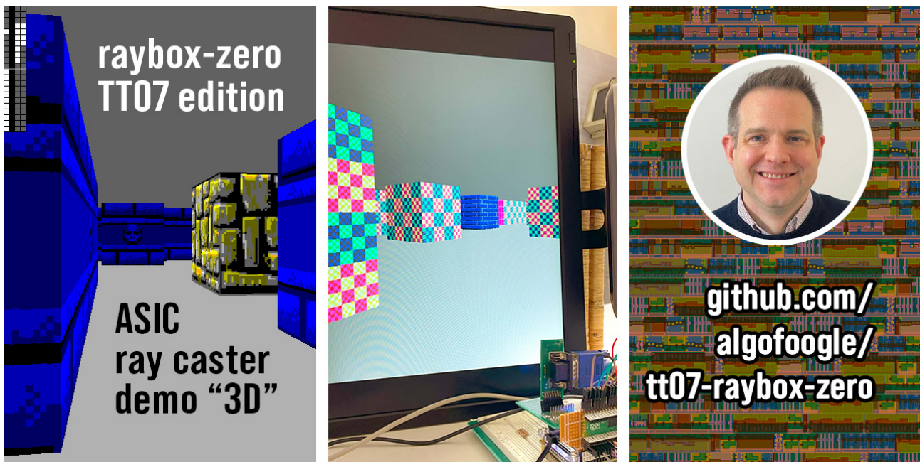
Figure 43: TT07 raybox-zero showing 3D views in simulation and on an FPGA
